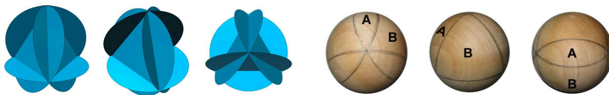
Fig. 9: Overlapping shell segments of the 3^{\text{rd}} spherical harmonic ‘note’ [8].
